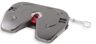
Specifically designed with safety in mind, this three-sensor safety system was the first of its kind to alert a driver from inside the cab as well as during the coupling procedure. Being constantly monitored, the system uses warning lights and a buzzer to alert any misscoupling or tampering. Camis is now manufacturing and supplying these units in increasing numbers.
